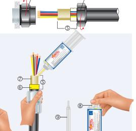
7. Re-insert the barrier pot sub-assembly \$\begin{aligned} \text{ back into the nipple nut } \text{ 2}.
