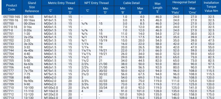
All dimensions except NPT are in mm. Intermediate thread sizes are available on request. NPT threads should be tightened 'wrench tight'.
