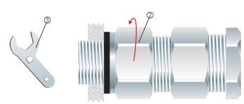
Screw the gland unit into the apparatus. Tighten the inner  $\ensuremath{\mathbb{Q}}$  to the installation torque using a CCG Spanner 5.
