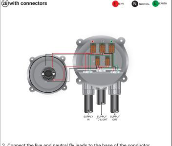
2. Connect the live and neutral fly leads to the base of the conductor connectors as indicated above.
