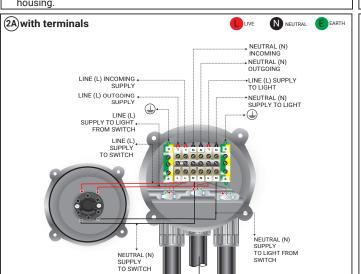
2. Use a terminal screw driver to connect the live and neutral fly leads to the base of the terminals as indicated above.
