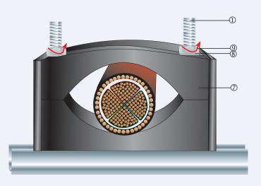
3. Slide upper shell O and washers  $\circledast$  over top half of the T-Bolts O and tighten nuts  $\circledast.$
