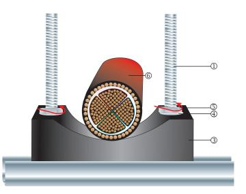
2. Place washers 9 on the T-Bolts 1 and tighten with nuts 5. Lay cable 6 in lower shell 3.
