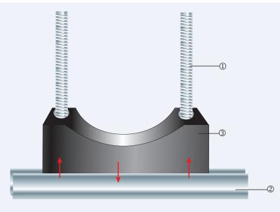
1. Slide both T-Bolts  ${f 0}$  through the rail  ${f 0}$  and then slide lower shell  ${f 3}$  over bolts as indicated.
