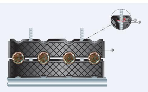
3. Slide the upper block part ® and washers ® over the top half of the T-Bolts ® and tighten the nuts ®.
