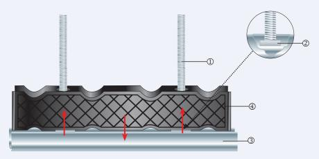
1. Screw the T-Bolt ① into the washer ②. Slide both T-Bolts ① through the rail ③ and then slide lower block part ④ over bolts as indicated.
