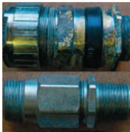
Image 1: 4 microns of nickel plating, Image 2: 12 microns of nickel plating
