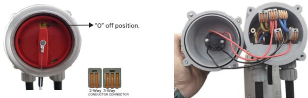
1. Remove the switch assembly by loosening the screws on the switch housing.
