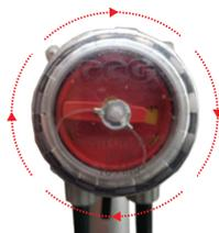
6. Hand tighten the dust cap.
