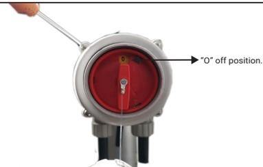
4. Ensure that the four screws on the switch housing are tightened to maintain IP66.
