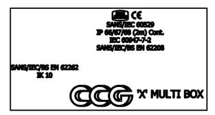
MARKING TO BE MOULDED OR ENGRAVED ONTO BOX COVER
